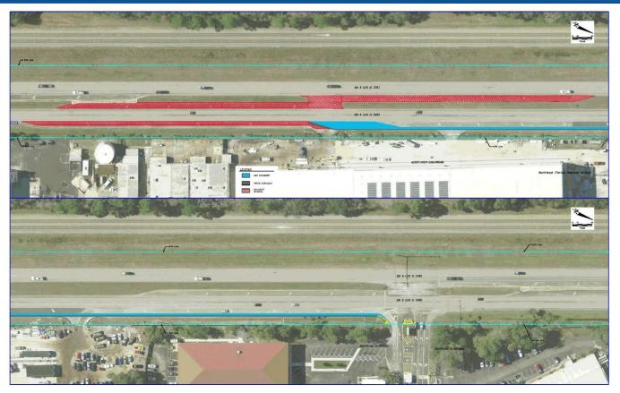
The double-stacked graphic above depicts the extents of pavement removal and the location of the Northrop Grumman entrance. The top portion displays the proposed modifications.
